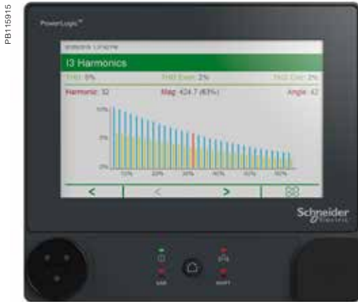
PowerLogic ION9000 Harmonics display
