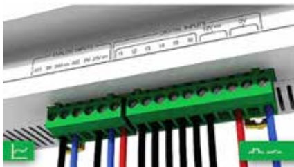
Power supply to analogue and digital inputs
